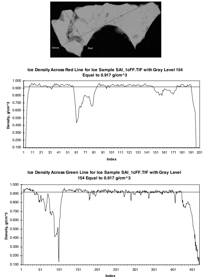
Fig. 8 Sample SAI 1cFF.TIF for the glaze ice case; V = 150 \text{ mph} , \text{LWC} = 1.0 \text{ g/m}^3 , \text{MVD} = 20 \text{ }\mu\text{m} , T_{\text{tot}} = 28^\circ\text{F} , and \tau = 12 \text{ min} .
