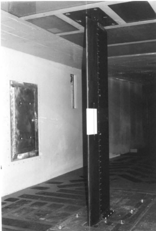
Fig. 2 NACA 0012 airfoil at a 0 -deg angle of attack, positioned for testing in the IRT. The white patch in the center of the airfoil is the electric heater.
